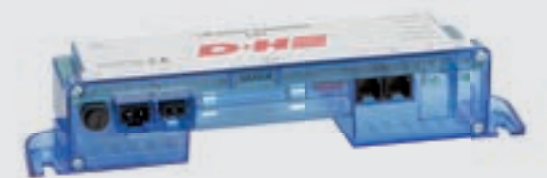
Lift status transmitter: Equipped with an integrated temperature, air quality and acceleration sensor
