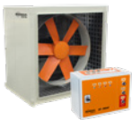
39 KIT BOXSMART Pressurisation system for stairs or evacuation routes. Maintains a differential pressure of 50 Pa in a single stage, designed according to the European standard EN 12101-6
