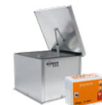
48 KIT BOXSMART FLAP Pressurisation system for stairs or evacuation routes. Maintains a differential pressure of 50 Pa in a single stage, designed according to the European standard EN 12101-6
