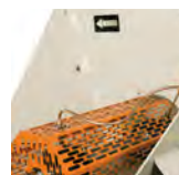
External greasers for ease of maintenance
